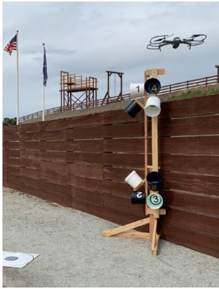
The WALL test shown with alternating pairs of white and black buckets to increase the need for exposure control.
