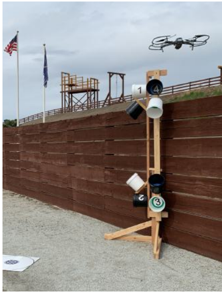
The WALL test shown with alternating pairs of white and black buckets to increase the need for exposure control.
