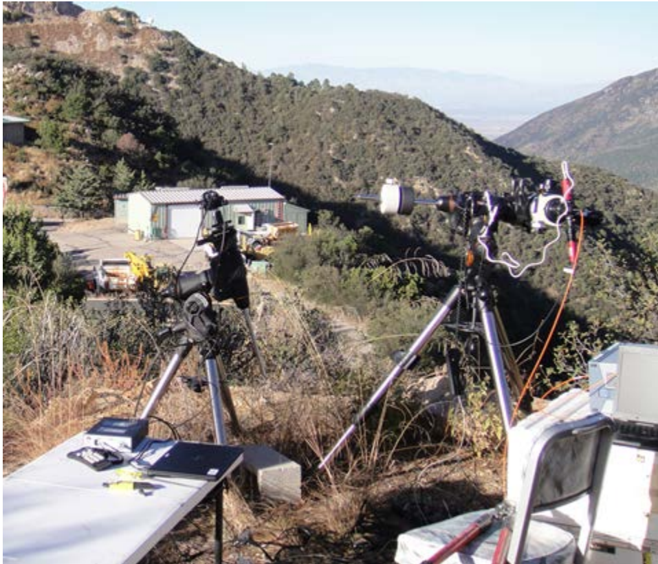
Figure 4. The observing telescope (right) and collimated laser for horizontal extinction (left) on the ridge at Mt. Hopkins. The calibration source was located in the support building in the background.
