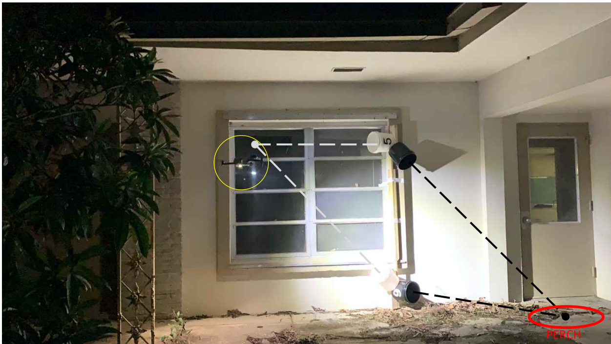
Figure 34). Obstructed test apparatuses embedded into an exterior house search at night show the designated hover positions and orientations including a perch position in view of the back door. The aircraft was outfitted with lights to illuminate the scene but also used its thermal vision capabilities to negotiate the myriad of obstacles such as trees, power lines, shrubs, etc.
