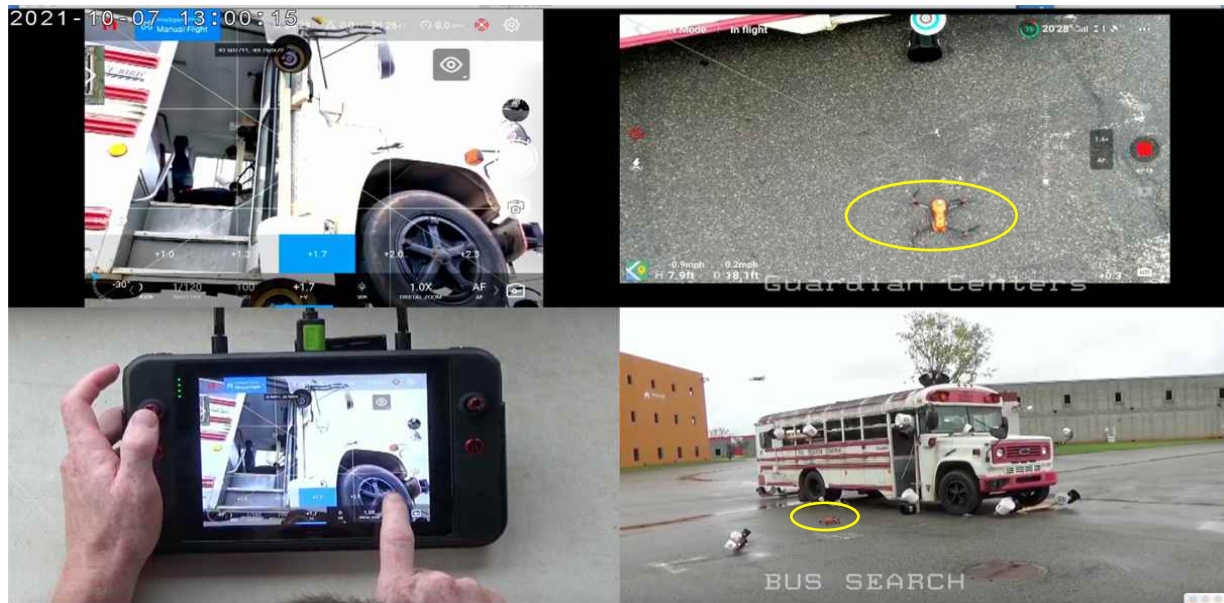
Figure 17) The quad screen video of the bus hostage scenario showing the drone point of view in the perch position (upper left).
