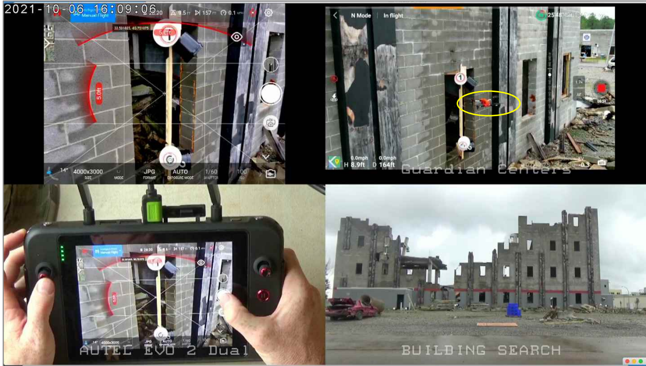
Figure 28) Our quad screen video captures simultaneous views of a trial, including what the remote pilot sees through the interface, all interactions with the interface, and off-board views showing the situation around the aircraft.
