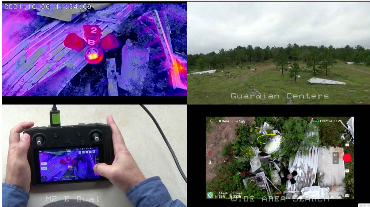
Figure 11) Quad screen trial videos capture the following concurrent views. TOP LEFT: The pilot's interface showing the thermal identification of a hand warmer inside an black omni bucket stand to represent a partially exposed survivor within the wreckage. BOTTOM LEFT: All operator inputs to the system. TOP RIGHT: An overview of the scenario. BOTTOM RIGHT: A detailed view of the drone in proximity to the objects of interest.
