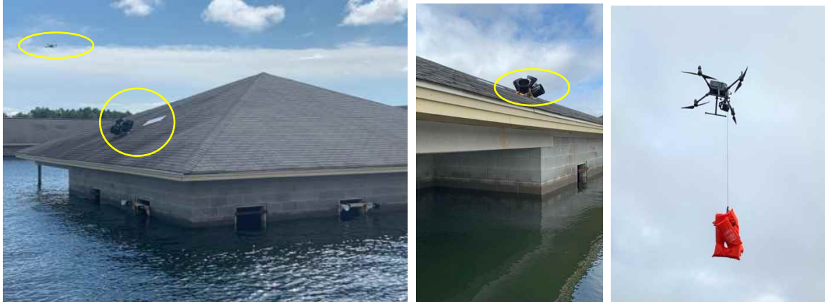
Figure 30) Victims on the rooftop of a flooded house were replaced with omni bucket stands to perform identification tasks and a landing was used as an accuracy target for dropping a personal floatation device.
