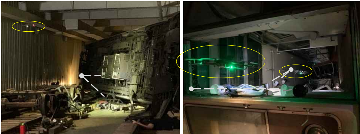
Figure 39) LEFT: We used Confined dual bucket alignments to designate 10 positions and orientations outside the subway car where victims were located along with suspicious packages. RIGHT: Two drones flew in tandem to help one another with side views of their situations as they negotiated the complex interior of the overturned railcar.
