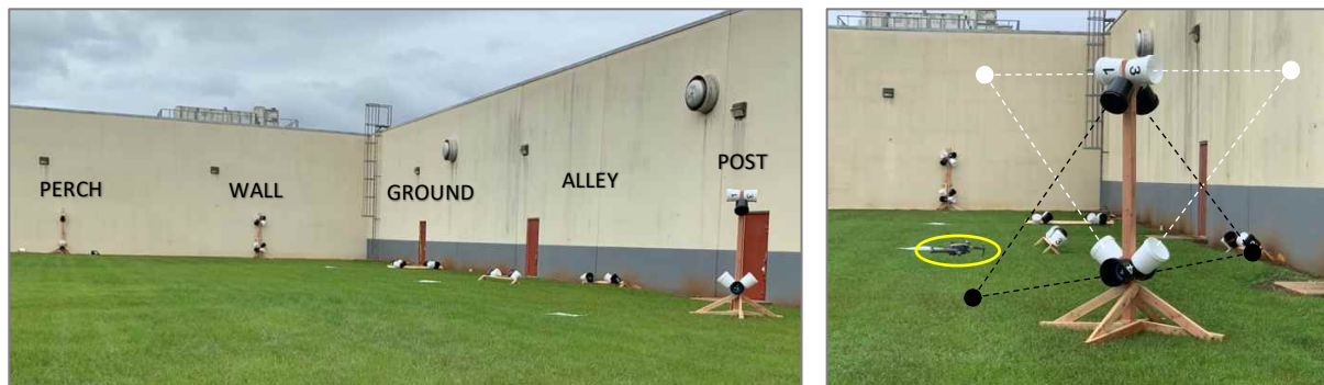
Figure 13) LEFT: The Obstructed Test Lanes are typically set up in order of increasing difficulty left to right as Perch, Wall, Ground, Alley, and Post. RIGHT: The Post test shown requires circumnavigating all the way
