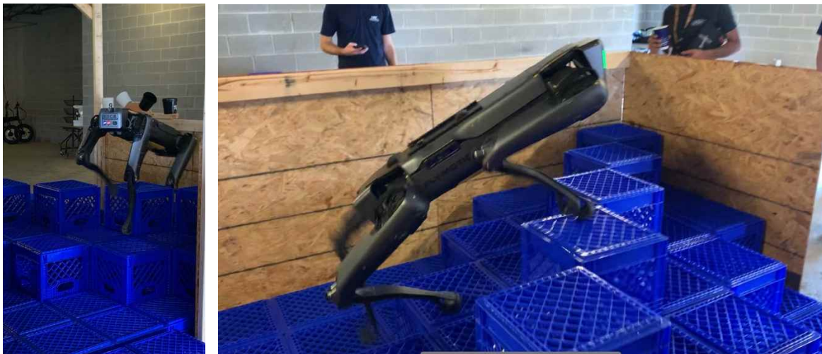
Figure 43) The Boston Dynamics Spot without its manipulator or extra sensors practicing the crate terrains.
