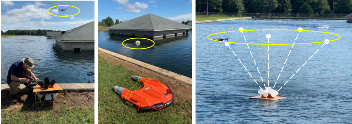
Figure 32) A floating omni bucket task was pulled through the water by a remotely controlled rescue device to represent floating or swimming victims. It provided a moving object for the drone to identify on all sides.
