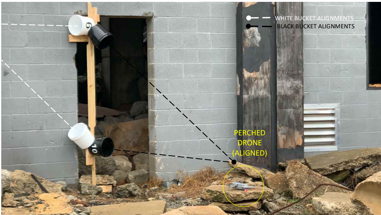
Figure 29) This final vertical test apparatus leads the remote pilot to perch with a view through the doorway. This was the 10 th and final position and orientation in the scenario that totaled up to 100 points for a complete search through the windows of the façade on two sides of the structure.
