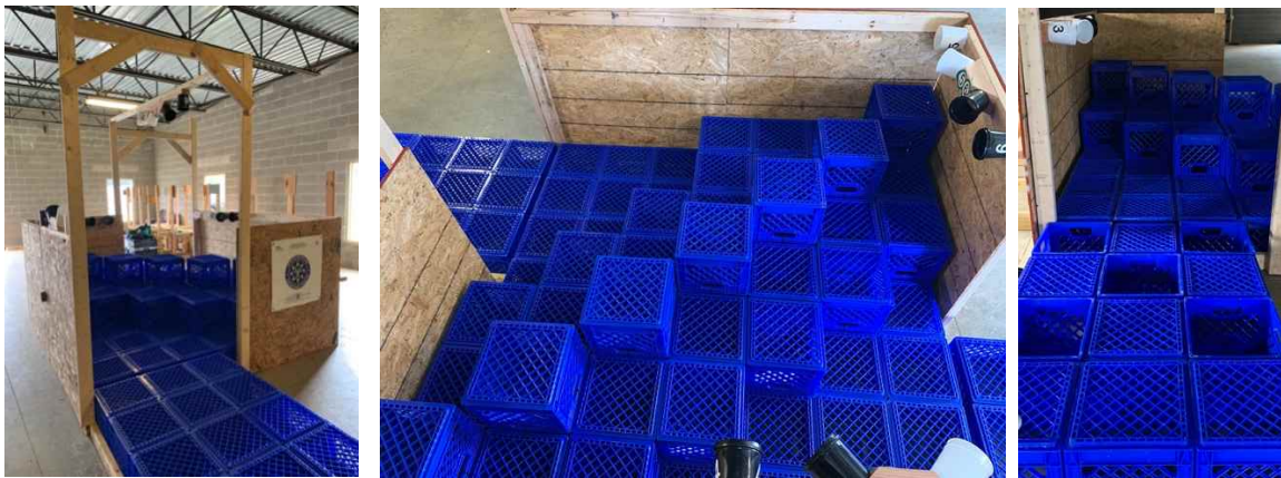
Figure 42) LEFT: The zig-zag crate terrain is easy to reconfigure for increasingly difficult challenges. CENTER: The diagonal hill with no holes. RIGHT: The checkered version of the terrain with holes either to avoid or deal with.
