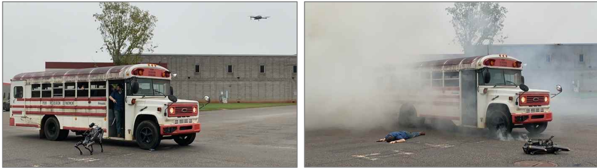
Figure 14) LEFT: One drone dropped a mobile phone to establish communications while another surveilled the situation. RIGHT: The ground robot also supported interactions prior to tactical intervention by law enforcement officers.
