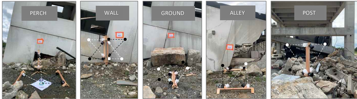
Figure 35) The Confined Test Lanes are half the size of the Obstructed Test Lane but use all the same procedures and scoring. They are typically placed near related scenarios such as this semi-collapsed building and parking decks with interior room-to-room searches and other confined space inspections. LEFT TO RIGHT: Perch, Wall, Ground, Alley, and Post tests evaluate positions, orientations and perches within 1 m (3 ft) of objects to identify features.
