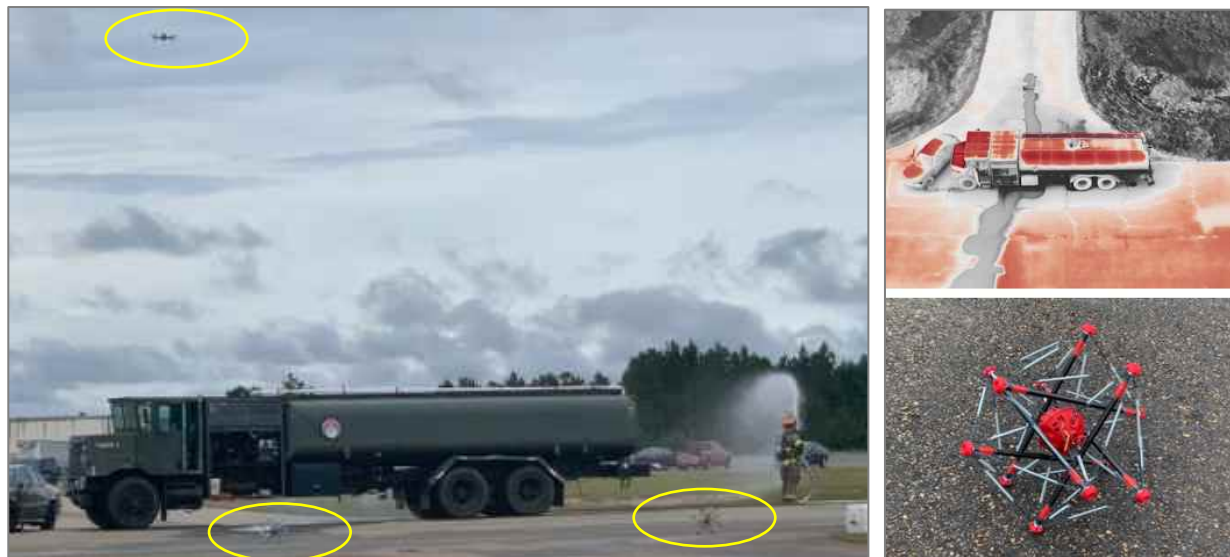
Figure 23) LEFT: The tanker accident scenario included a simulated fire and potential hazmat spill requiring firefighters to react as appropriate based on reconnaissance from the drones and dropped sensors. RIGHT: Thermal overview image from the drone and the dropped sensor packages.
