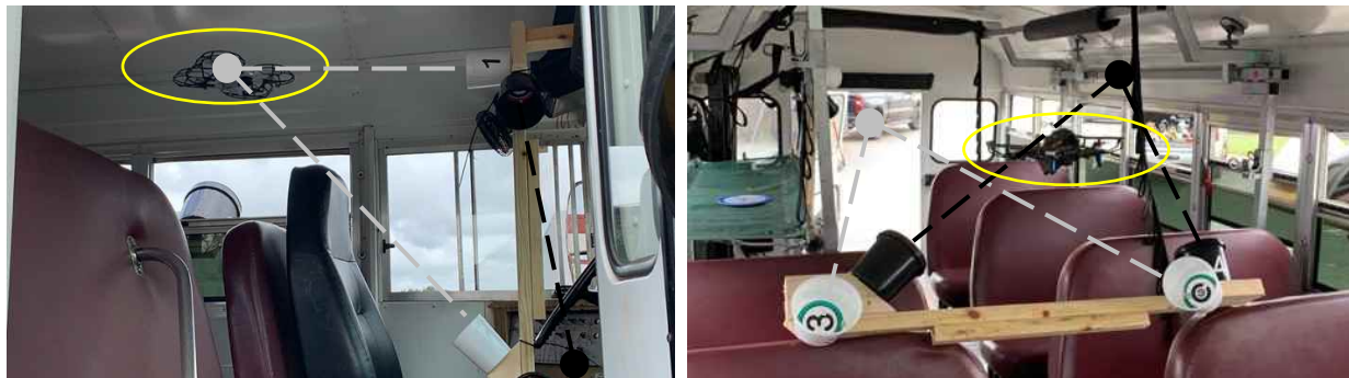
Figure 18) LEFT: An interior dual bucket alignment (buckets 1 and 1A) just inside the entry door at the driver's seat. The perpendicular (90 degree) bucket provides a safe vector to approach the apparatus until the angled bucket (45 degree) is simultaneously aligned. That's the safe 1m (3ft) standoff position at which the pilot should maintain position knowing the drone is safe from obstacles and work the interface controls for zoom, focus, and exposure to capture an image that can be scored after the trial. RIGHT: Other dual bucket alignments were related to views of objects on the seats, under the seats, and near the back door on the floor.
