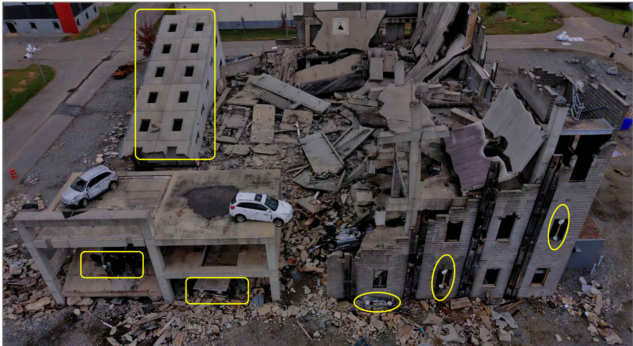
Figure 25) The collapsed structure had several different scenarios to fly. The Obstructed scenarios (some shown with ovals) were perimeter windows, doors, and surrounding ground objects. The Confined scenarios (some shown with rectangles) were vehicles in the semi-collapsed parking garage and room-to-room searches inside the semi-collapsed building.
