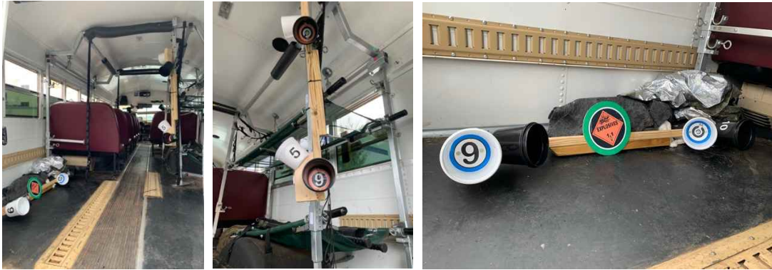
Figure 19) LEFT: Other interior tasks using the small buckets in confined search spaces. CENTER: Two apparatuses require vertical alignments. RIGHT: Three apparatuses require horizontal alignments. This is the final perch position to maintain a view of an object of interest.
