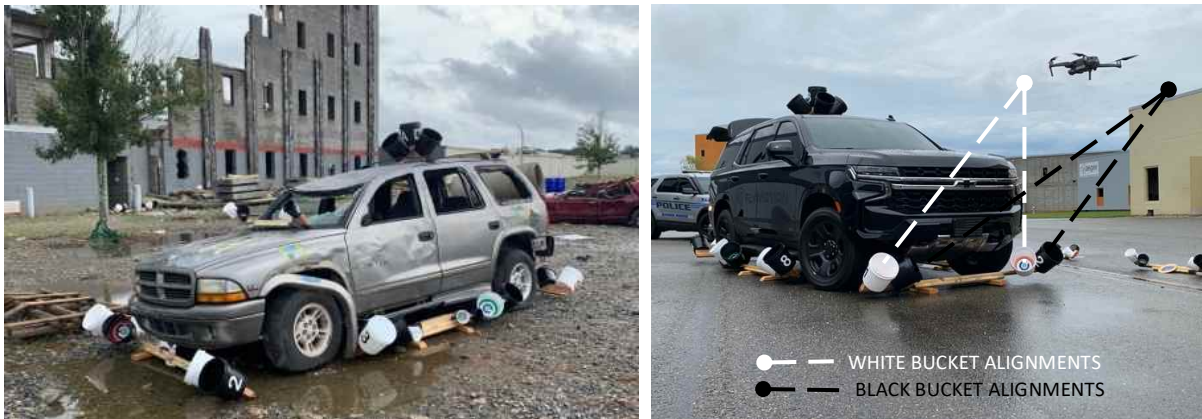
Figure 20) LEFT: Vehicles of all sizes and conditions can be bucketized similarly for quantitative scoring, including panel vans and trucks. RIGHT: Dual bucket alignments guide the drone into position to look inside the front windshield from two different angles while using triangulation between the buckets to stay safe.
