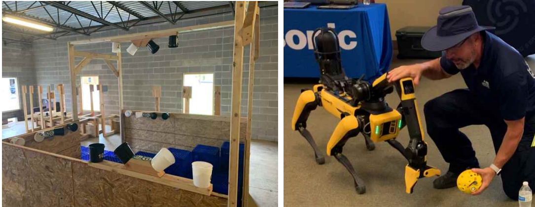
Figure 44) LEFT: Embedded search/inspect tasks with dual bucket alignments that measure the difference between robots with and without manipulators that can position, orient, and zoom cameras while negotiating various terrains. The search/inspect tasks are exactly like the aerial Confined Test Lane tasks but require a closer 30 cm (12 in) standoff position to align with each pair of buckets simultaneously. RIGHT: Fetch tasks may be the next set of tests to standardize!
