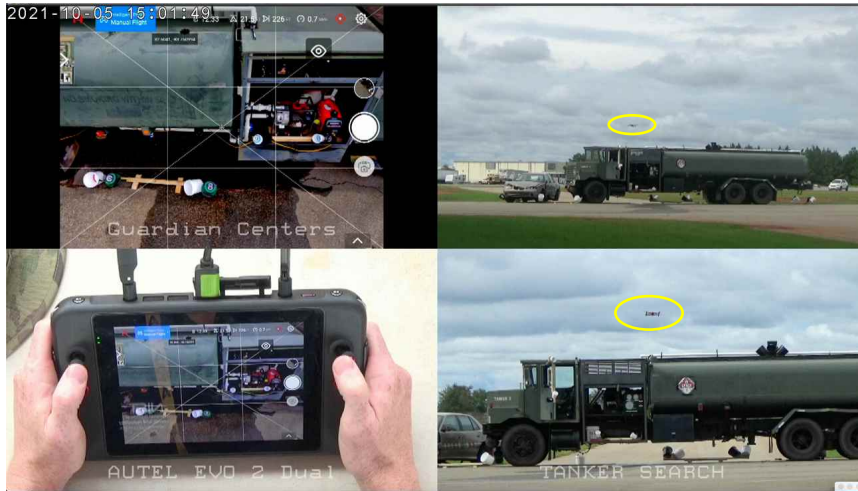
Figure 24) Our quad screen video captures simultaneous views of what the remote pilot sees through the interface, all interactions with the interface, and off-board views of the situation around the aircraft.
