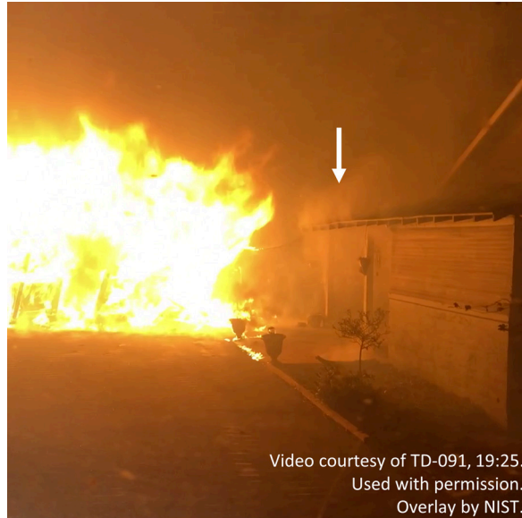
Figure 58. Fully involved shed, 8 m × 4 m (13 ft × 26 ft), located 3 m (10 ft) from the primary structure. Eaves of the primary structure are pyrolyzing (white arrow).
