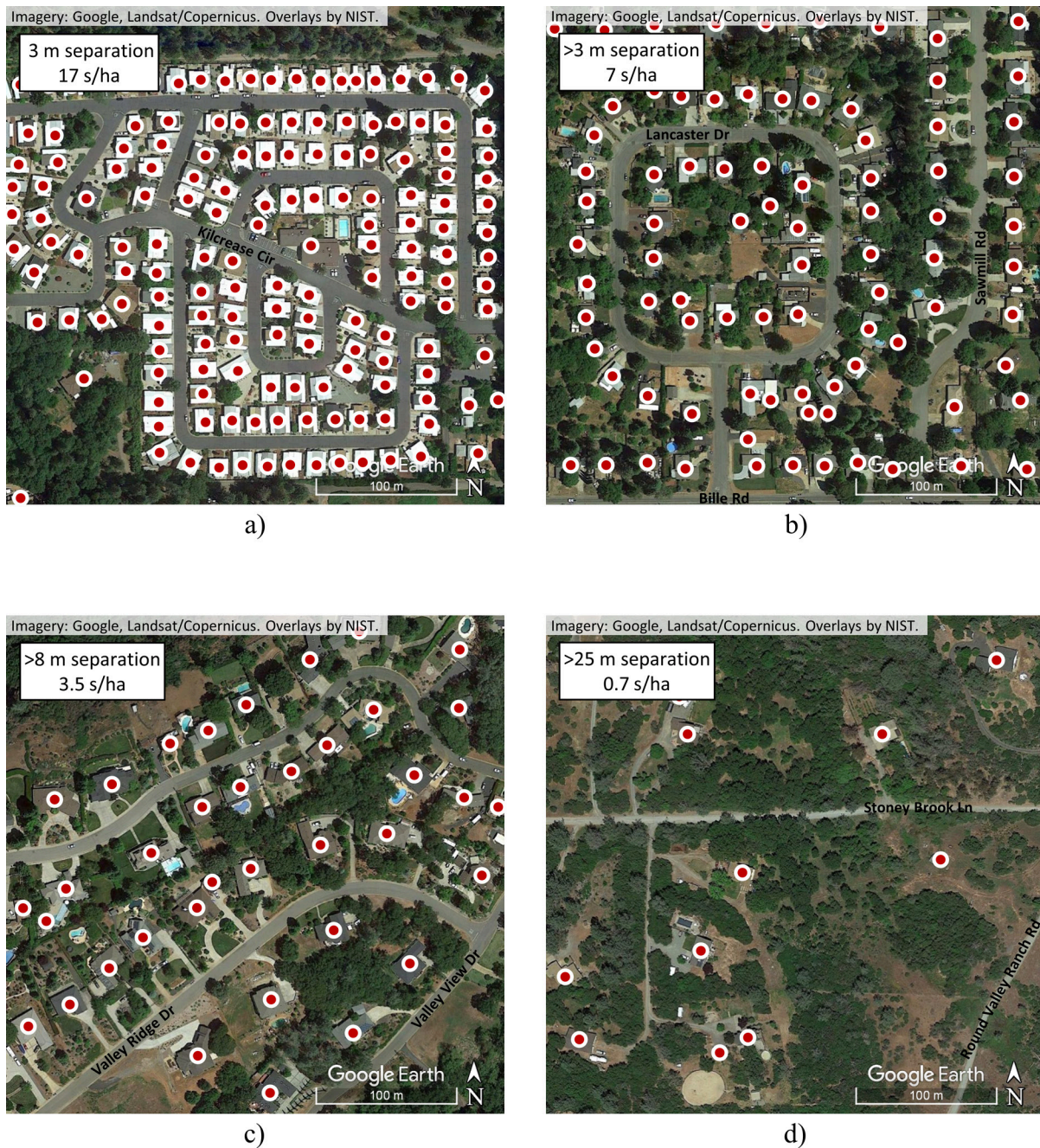
Figure 2. Homes within Paradise display a wide range of structure-to-structure separation. Representative images show progressive reductions in structure density from locations; a) Apple Tree Village Mobile Home Park, b) Lancaster Dr, c) Valley Ridge Dr, and d) Round Valley Ranch Rd. Also note the variability in vegetative fuel density.
