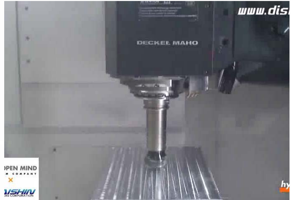
5-Axis Machine Cutting of Helmet (Daishin Seiki Corporation)
