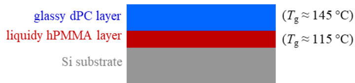
Figure 2. Schematic of the bilayer samples. When the sample is annealed at 140 - 150 °C, the d PC is in the sluggish glass transition state and the h PMMA is in the liquidly melt state.
