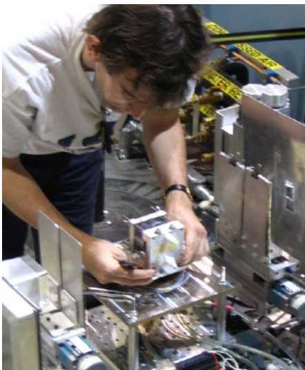
Duncan McGillivray aligns the NCNR wet cell.
