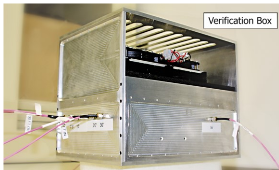
Multipath verification artifact (conducted channel)
