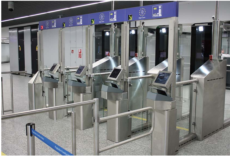
Figure 2: EasyPASS hardware setup - four operating eGates in parallel
