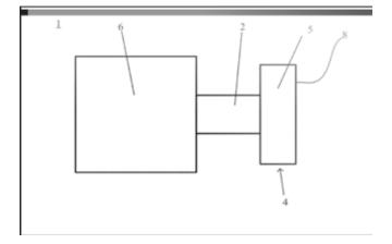
Optical meter 1 includes ref ector 4 disposed force member 2. Ref ector 4 is conf gured to receive radiation and to communicate a pressure of the radiation to force member 2. Ref ector 4 includes substrate 5 and ref ective surface 8. Force member 2 is conf gured to be displaced in response to receiving the force comprising the pressure, and optical meter 1 is conf gured to measure a power of the radiation, an energy of the radiation, or a combination thereof based on the pressure.
