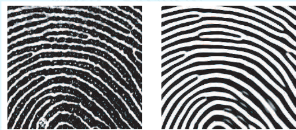
(a) Input image (1000 ppi) (b) Gabor enhanced image
