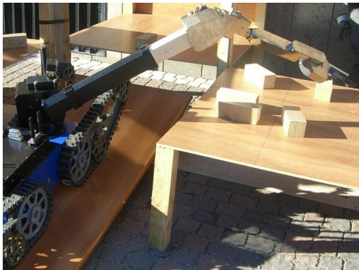
Fig. 4. Grasping Dexterity Test at 2006 RoboCamp Rome, Italy with teleMAX Bomb Disposal Robot
