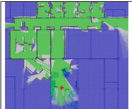
Figure 5: Competitors map overlaid on ground truth from an indoor scenario.
