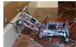
Fig. 4. Whegs robot with a body flexion joint surmounting a larger step than the robot's body height
