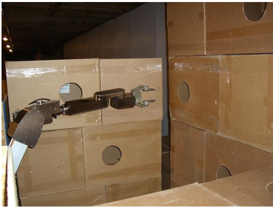
Fig. 3. Directed Perception Test at 2007 Metro Tech Event, NIST with teleMAX Bomb Disposal Robot
