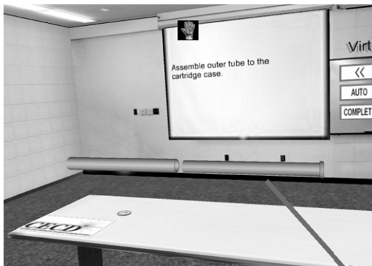
Fig. 3. An example of sub-type B2 symmetry where the attachable part (outer tube) can only be inserted at the primary position, but with either primary or alternate orientation (around the secondary axis). Secondary axis is perpendicular to the main axis, which is the axis of the cylinder.
