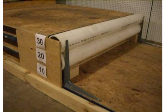
Fig. 6. NIST 30cm Step Test with Pipes
