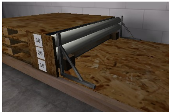
Fig. 7. NIST 20cm Virtual Step Test with Pipes
