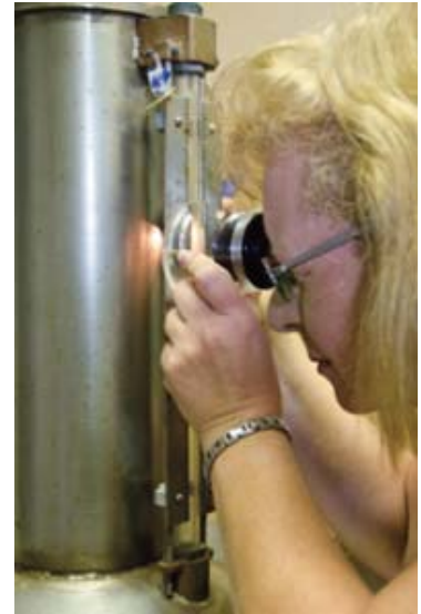
PML technician Sherry Sheckels uses a flashlight and magnification loupe to take exact water-level measurements on a stainless steel container.
