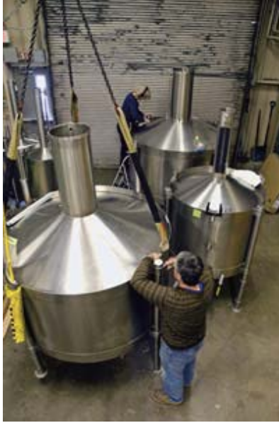
Two customers prepare their "cans" for calibration in PML's Fluid Metrology facility.
