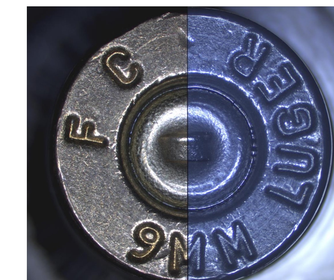
Comparison microscope image of a master casing (left) and replica (right)
