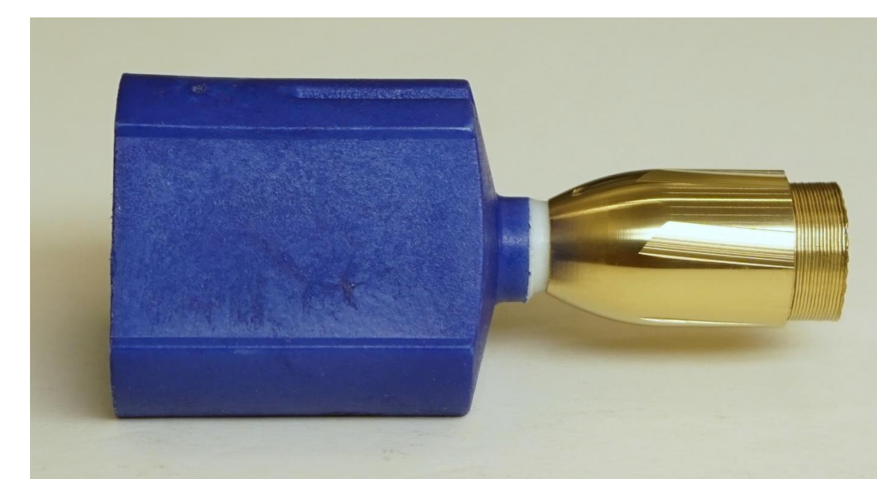
Gold coated replica on a sample holder
