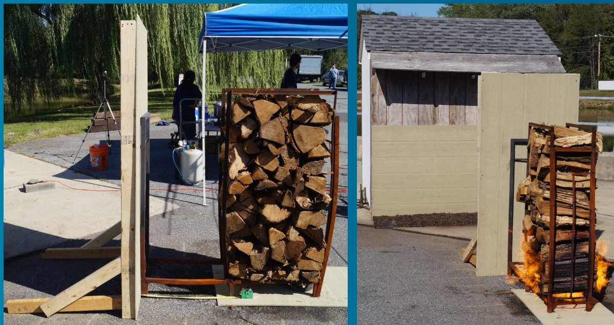
Wind/Ember Blocking Wall
