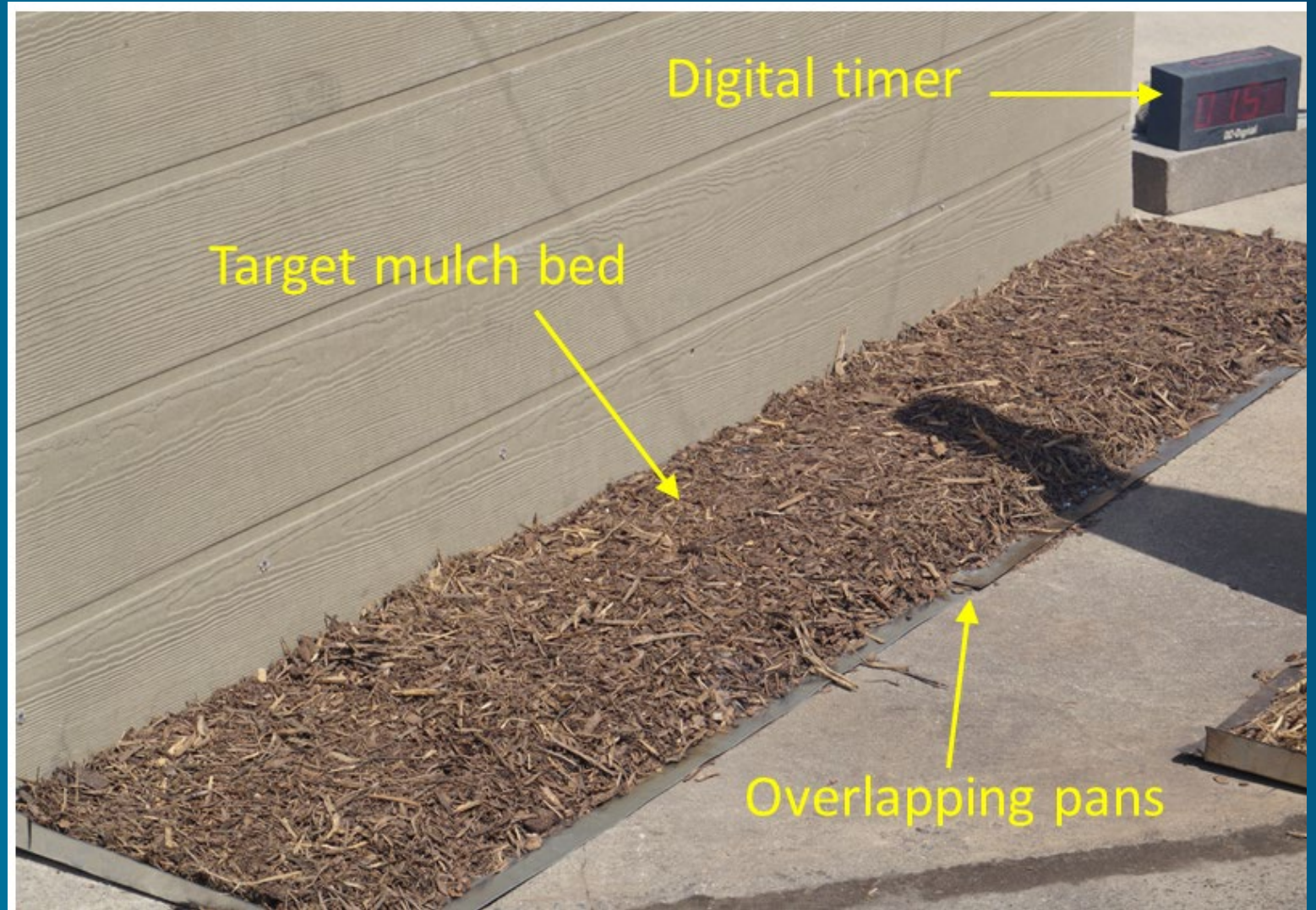
Structure (shed) + mulch at base
