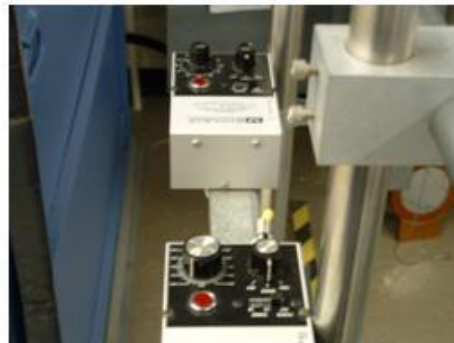
Chamber alignment controls 100 kV range
