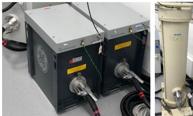
Figure 4b Voltage dividers, GE on left and Pantak on right.
