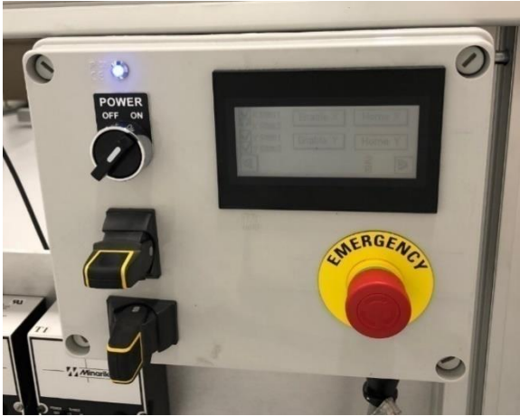
Hand control LPS motion controller with EMO button on telescope stand
