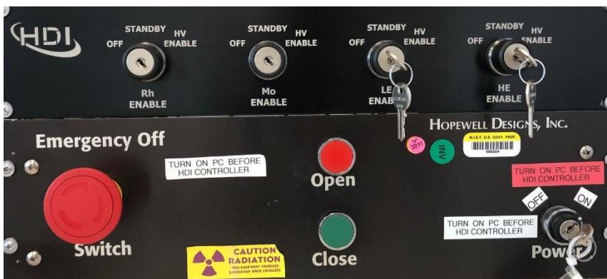
Figure 8a HDI controller and x-ray tube key interlock
