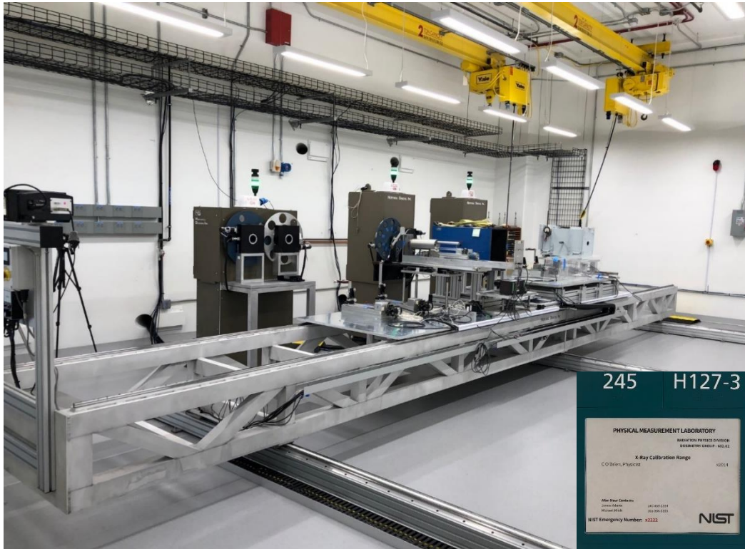
Figure 1 The NIST X-Ray Calibration Facility showing primary standards and the linear positioning system.
