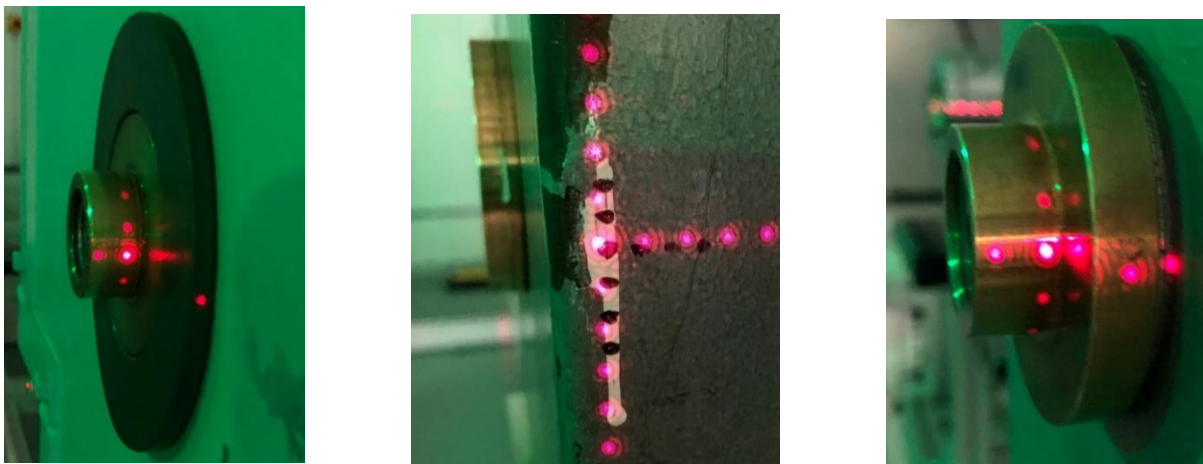
Figure 19 Alignment points of standards, showing laser crosshair.
