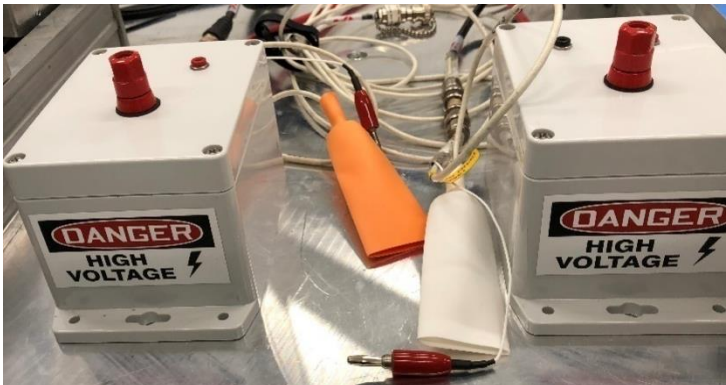
Figure 17 Test chamber voltage connection boxes.
