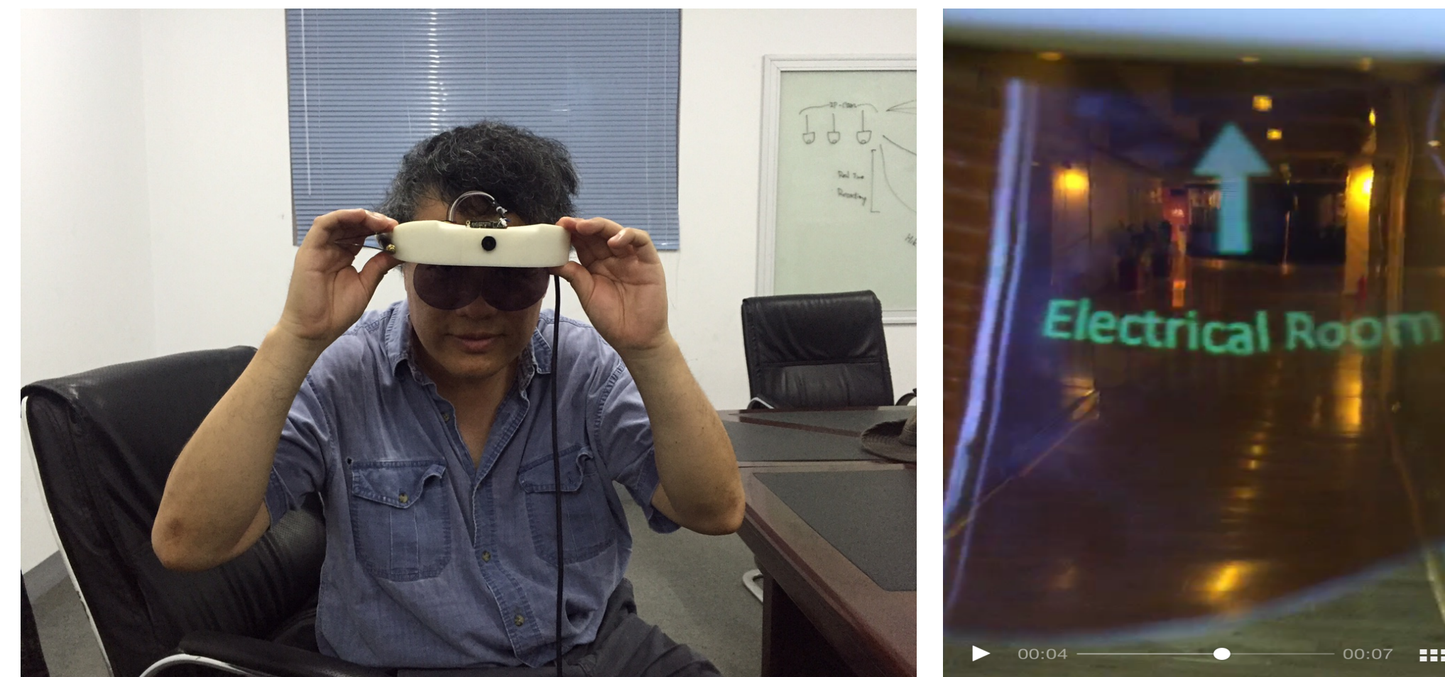
The prototype of the smart helmet (left) and the projected navigation information about where is the electrical room (right)
