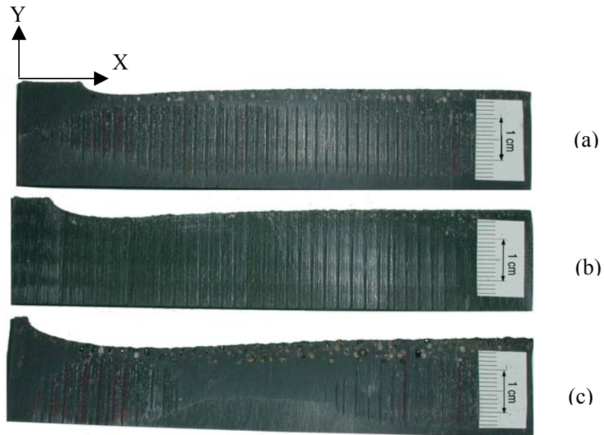
Figure 6: PMMA Surface profiles after (a) 5 min, (b) 10 min and (c) 20-min burns; Tests with 19.4% oxygen; flame spreading within X < 20 mm
