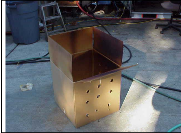
Figure 14 Class A fire load in hypoxic test
