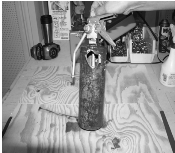
Figure 3.1.3-4 Entry and exit points—longitudinal axis of cylinder 45° toward gun position
