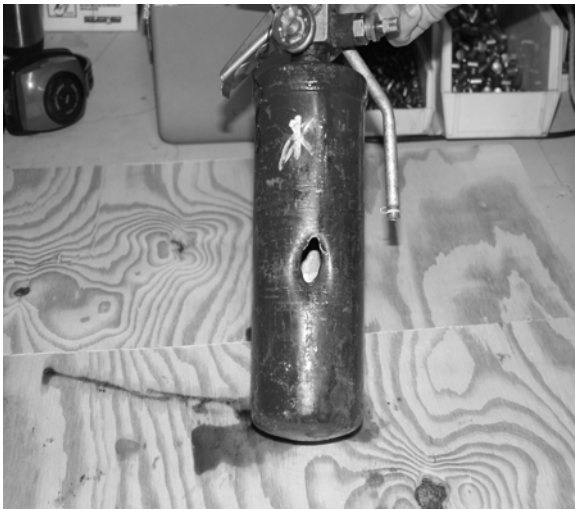
Figure 3.1.3-4 Entry and exit points—longitudinal axis of cylinder 45° toward gun position
