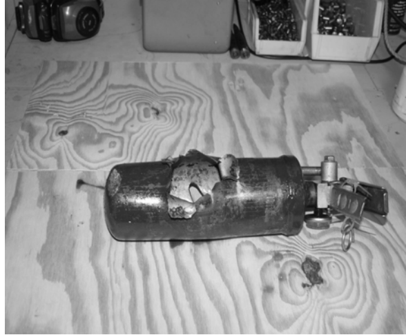
Figure 3.1.3-3 Entry and exit points – longitudinal axis of cylinder normal to line of fire
