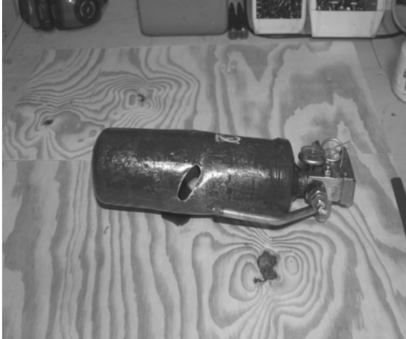
Figure 3.1.3-3 Entry and exit points – longitudinal axis of cylinder normal to line of fire
