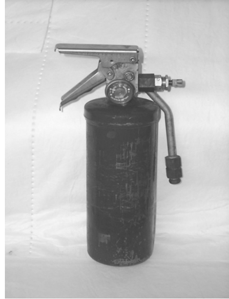
Figure 2.2-5 Modified valve assembly and experimental prototype
