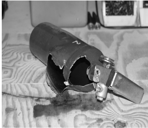
Figure 3.1.3-5 Entry and exit points – longitudinal axis parallel to line of fire
