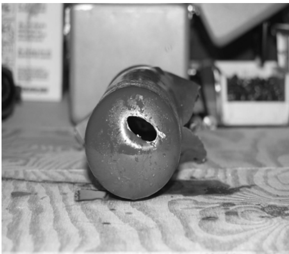
Figure 3.1.3-5 Entry and exit points – longitudinal axis parallel to line of fire
