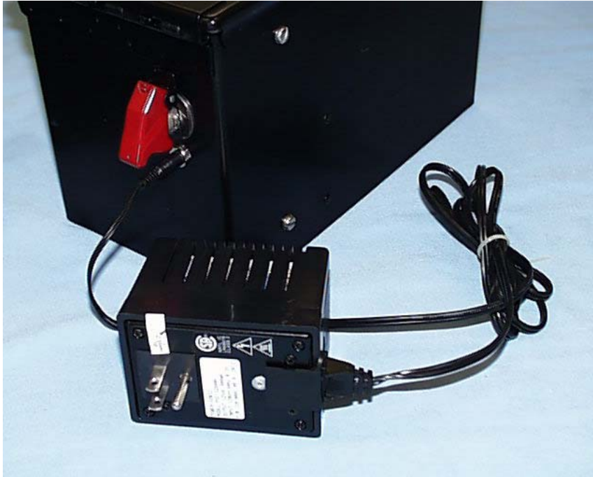
Figure 6. External charger and switch of the sequential sampler.
