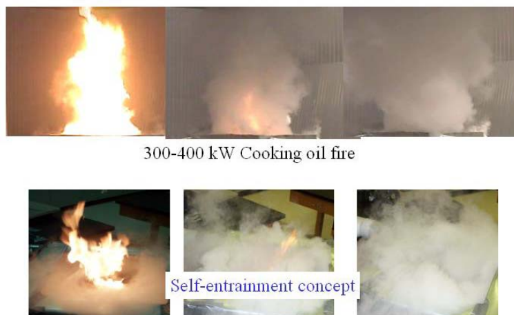
Figure 3: The gas-like UFM being entrained to the firebase of 300-400 kW cooking oil fires in deep fat fryer
