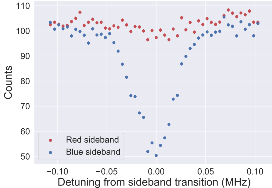
Figure 4.17: Verification of ground-state cooling of the out-of-phase axial mode with Raman beams. We scan across the sideband transitions after cooling the mode, exciting the blue sideband but not the red. This asymmetry indicates that the mode is close to its ground state (Eq. 4.11).
