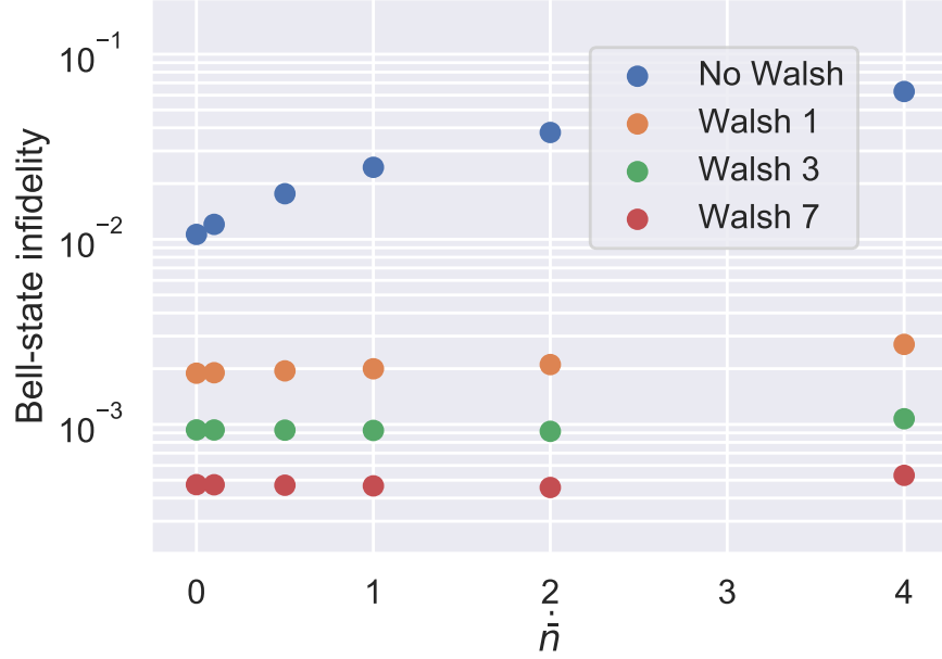
Figure 2.7: Simulations of Bell-state infidelity for a fixed detuning error versus temperature for different Walsh sequences. The detuning error is 200 Hz, with \Omega_g/2\pi = 1.25 kHz for all gates. Walsh modulation significantly reduces the temperature dependence of this error.
