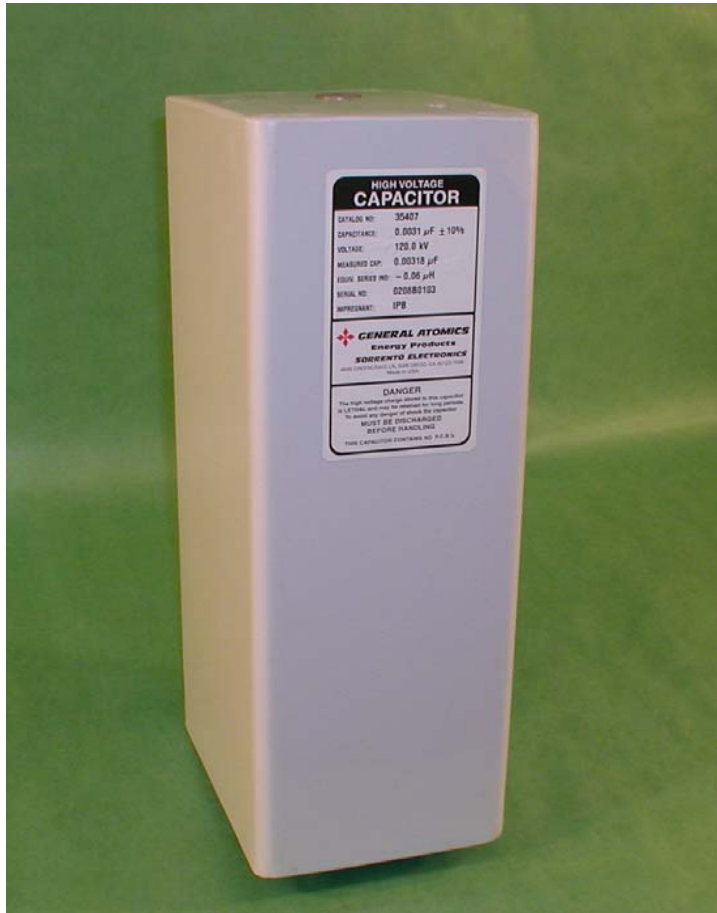
Transformer Resonating Capacitor 3100pF, 120kVDC, 85kVAC, 3.5 MVAR (Composite Dielectric)
