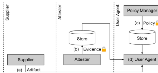
Figure 1 - Supply Chain Integrity Model - Overview
