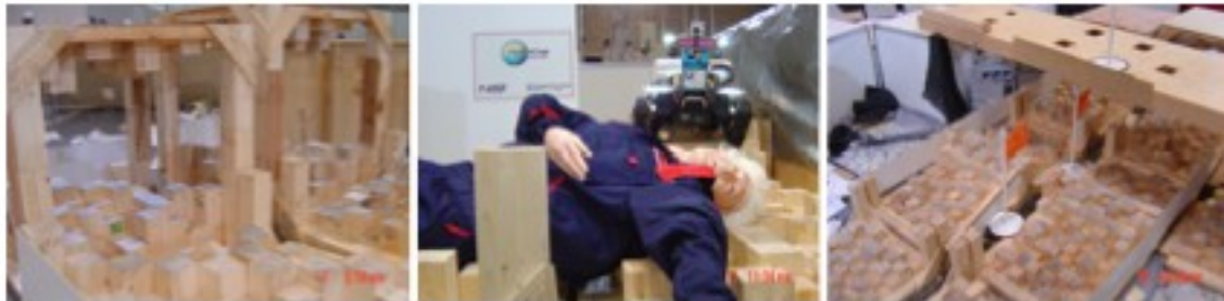
Figure 3: Recently developed random step fields were used within the arenas to provide well-defined mobility challenges. And as always, simulated victims emitting various signs of life (human form, heat, sound, motion, and/or CO 2 ) provided the incentive for robots to search the arenas in their entirety.
