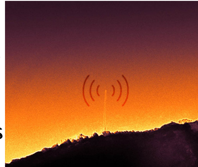
This image, taken by a transmission electron microscope, shows the carbon-nanotube radio (UCB)
