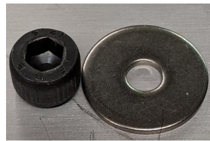
Fully successful fastener operation. Washer cannot be inserted under head. (3 points)
