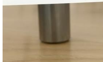
Full insertion with peg seated on surface that supports the task board (5 points)
