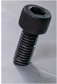
Cross threaded screw cannot advance thread by hand (no points)
