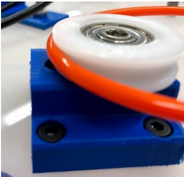
Lack of tension (no points)
