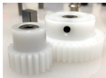
Both gears inserted and fully seated (5 points) for each.
