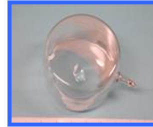
3 He neutron spin analyzer [W.C. Chen et al., Physica B, 404, 2663 (2009) ]
