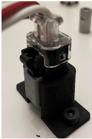
Insertion into mating counterpart and snap fit of locking mechanism (5 points)
