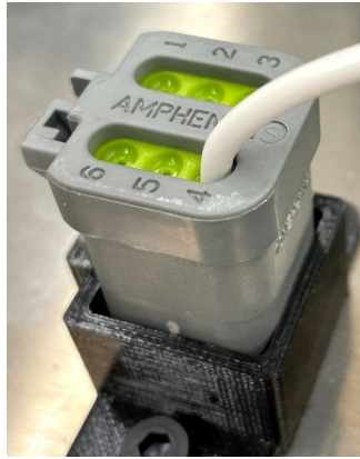
Inserted and fully seated. Cannot be removed with a tug. (5 points)
