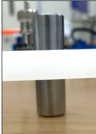
Full insertion with peg seated on surface that supports the task board (5 points)
