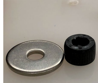
Fully successful fastener operation. Washer cannot be inserted under head. (3 points)
