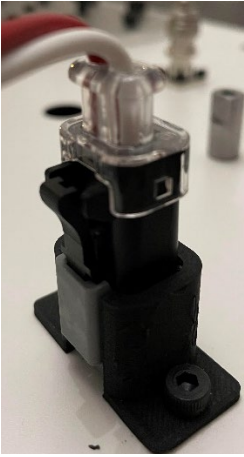
Insertion into mating counterpart but no snap fit of locking mechanism (3 points)
