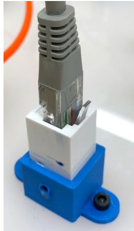
Insertion into mating counterpart and snap fit of locking mechanism (5 points)
