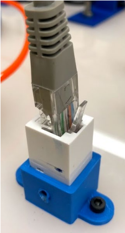
Insertion into mating counterpart but no snap fit of locking mechanism (3 points)
