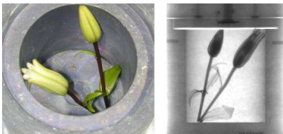
Figure: Flower in lead shielding showing the sensitivity of neutron imaging to hydrogen. (NIST)
