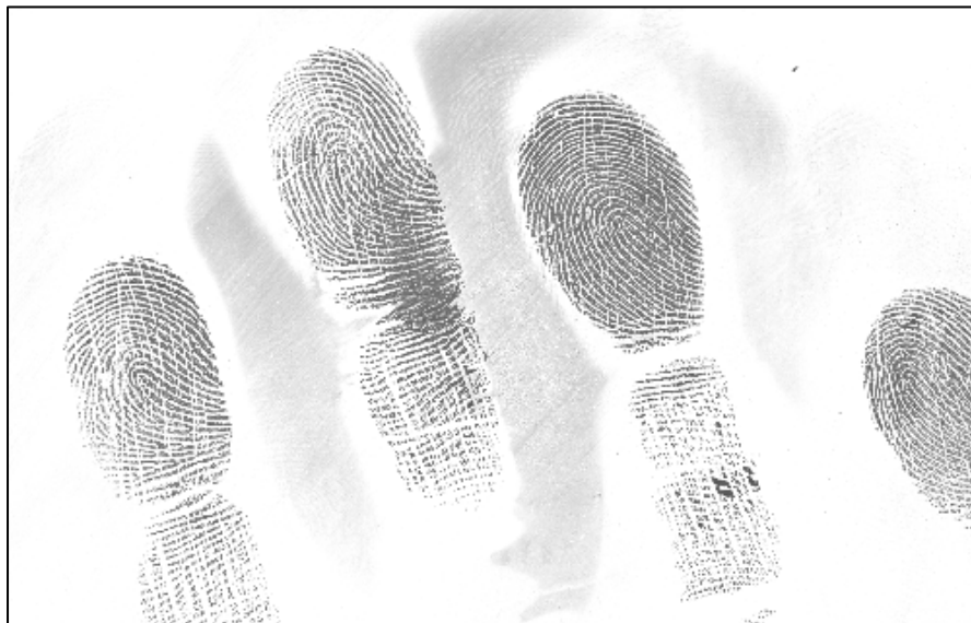
Figure 4. Moisture/Condensation on the platen surface.
