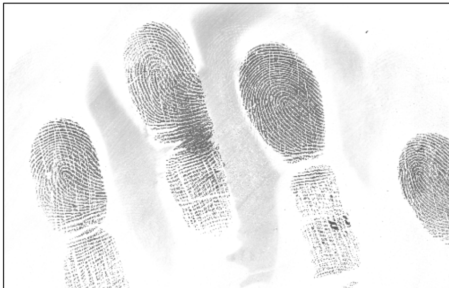
Figure 4. Moisture/Condensation on the platen surface.
