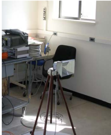
Fig. 17. Hardware experiment to validate the spatial spectrum generated by the ray-tracing tool.
