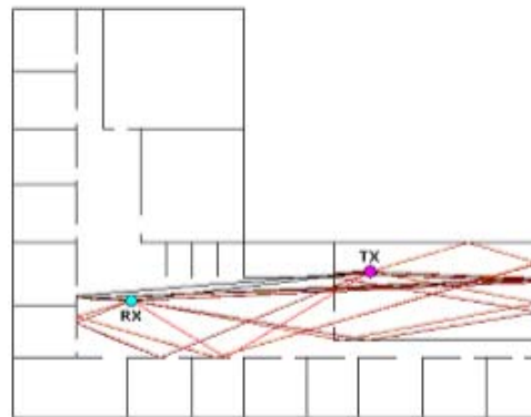
Fig. 5. Sample output of the ray-tracing tool for a given building layout.
