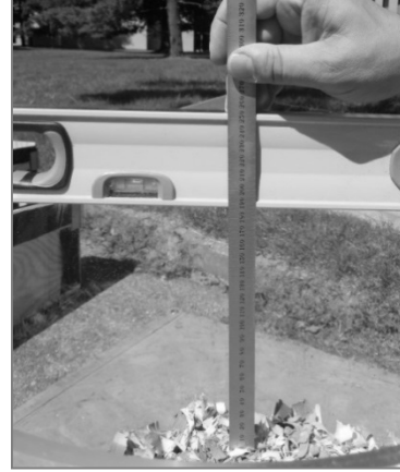
Figure 4. Showing how the ruler is placed on the bedding with the headspace method. The ruler is read from the bottom edge of a straight edge or level from a position that reduces parallax.
