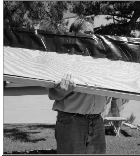
Exhibit 2. Showing how to cradle the chute on one arm and holding it with one hand while tilting it with the other hand.
