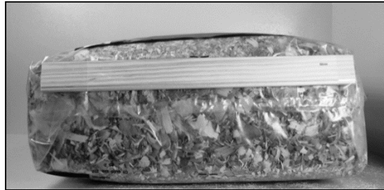
Exhibit 33. Plumped bedding package illustrating rounded edges (angles), which hinders getting accurate measurement points.
