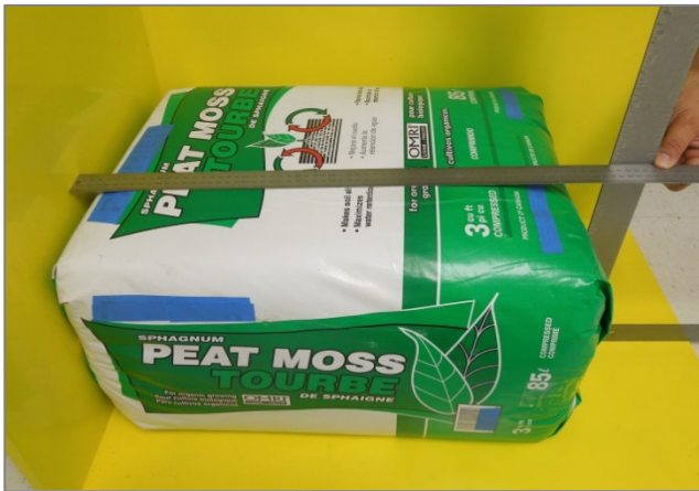
Exhibit 8. Height Measurement – A packaging tail on the end of the package can affect this measurement so it has been folded over and taped against the end of the package.
