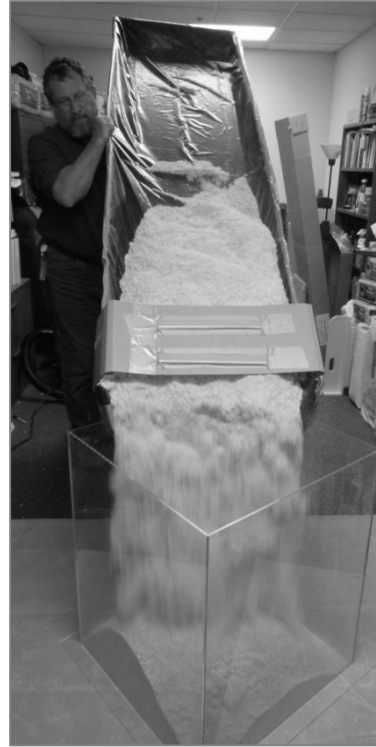
Exhibit 16. Filling a Square Test Measure at an Angle to use the Larger Opening.
