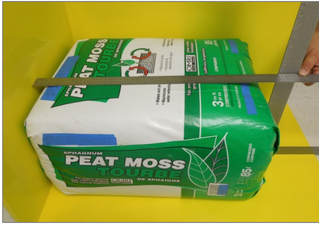
Figure 3-5. Height Measurement – A packaging tail on the end of the package can affect this measurement so it has been folded over and taped against the end of the package.
