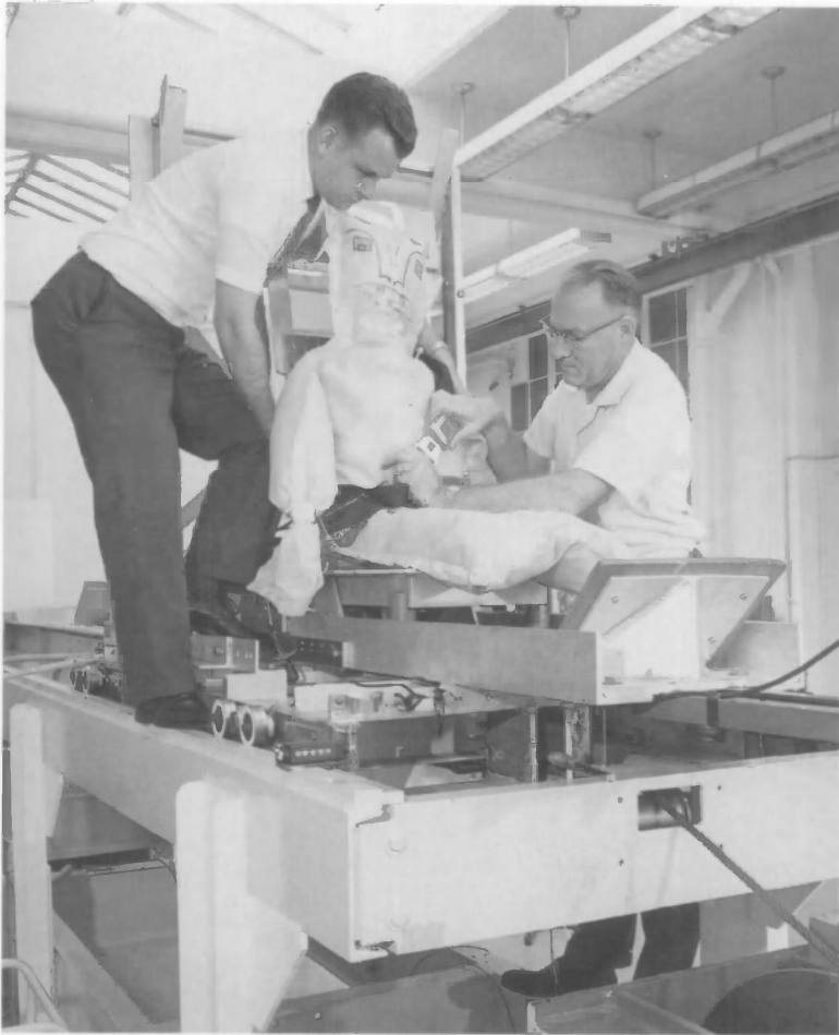
Robert Christian held "Sandy Bagg," as Earl Cooke belted Sandy in place on the sled of the NBS dynamic testing machine. Sandy was one of the contenders for the "standard dummy" for dynamic testing of automobile occupant restraint systems.
