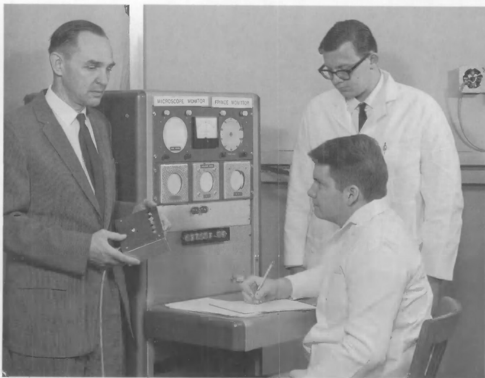
Herbert D. Cook (left) of the NBS Electronic Instrumentation Laboratory controlled the automatic operation of a fringe-counting interferometer (not shown). The count was shown on the monitor console (center).
