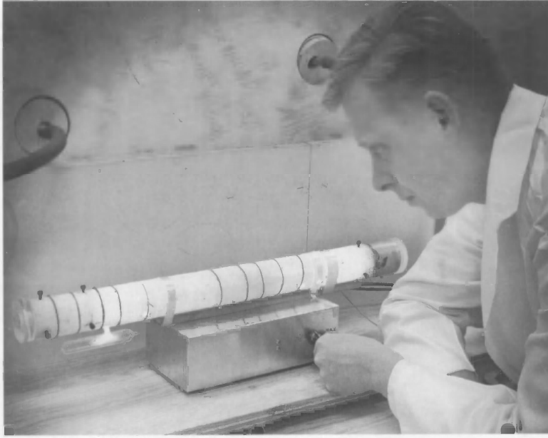
In the measurement of length with a laser to better than 1 part in 10 million, Klaus D. Mielenz matched the impedance of the rf-power supply to that of the laser.
