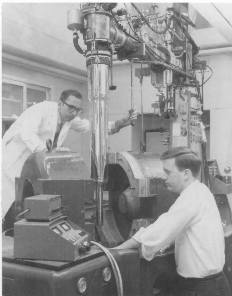
Earl R. Pfeiffer (left) and Calvin S. Koonce positioned a Dewar inside a magnet in preparation for an experiment to determine the superconducting transition temperature of strontium titanate as a function of conduction electron concentration.
