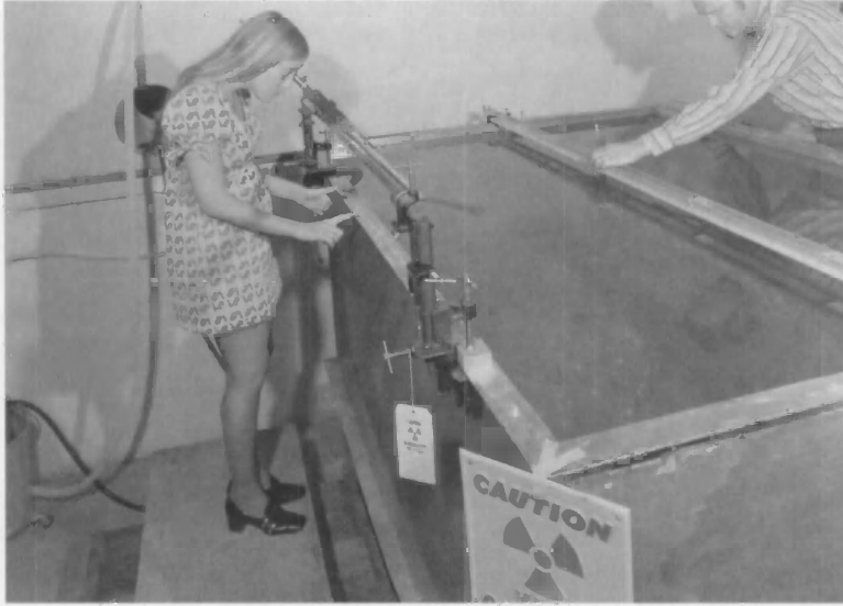
Valentine Spiegel, Jr. and his assistant Linda Cline determined neutron penetration depths in a water bath, using foil detectors positioned at precise distances from the source. After neutron activation, the foils were placed in a radioactivity counter to measure neutron fluence.
