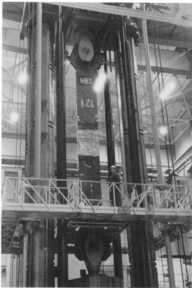
Mechanical Engineer Samuel R. Low stood on the platform of the NIST 12-million-pound-force Universal Testing Machine circa 1988. Behind him was the then-record fracture test specimen, a 35 ft long test specimen with a 6 in thick, 40 in wide insert. It took 5.94 million pounds of force in tension to fracture the insert.
