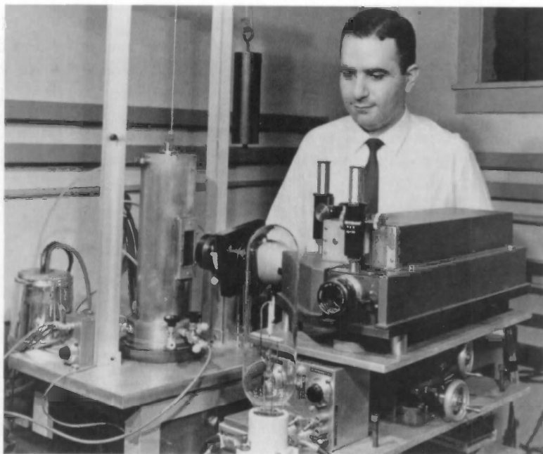
Physicist Ared Cezairliyan operated this apparatus to obtain high-temperature thermodynamic data in sub-second time intervals.
