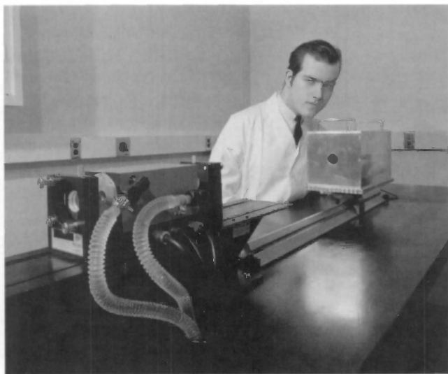
Arthur H. Neill, Jr. of the NBS Electronic Technology Division measured the output energy of a solid state laser, using a portable calorimeter that he developed in 1970.
