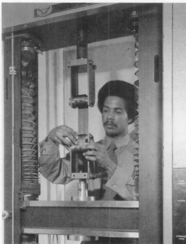
Dorian Sanders of the NBS Office of Vehicle Systems Research positioned seatbelt webbing in a tensile test machine. The resulting data was used to update Federal automotive standards in the early 1970s.
