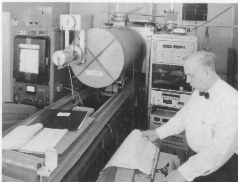
A digital printout of an emission spectrum from a soft-x-ray spectrometer was examined by its designer, John Cuthill. All optical and some mechanical components of the spectrometer were housed in the large cylinder (center). Data were recorded on a stripchart (left), on paper (foreground), and on magnetic tape (right) for input into a computer.
