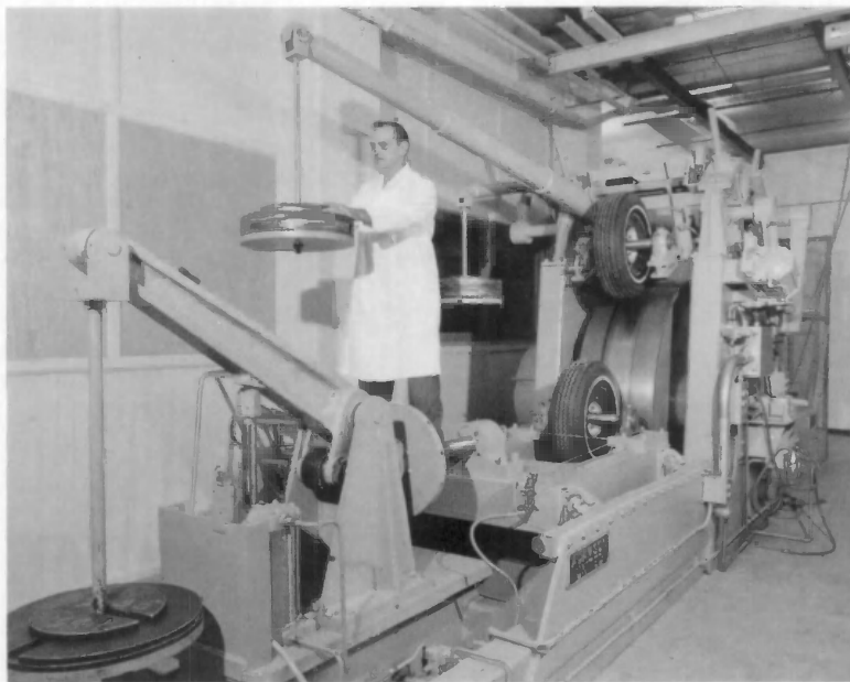
Tire endurance and heat sensitivity were tested on the “NBS Wheel,” a large wheel 1/300 of a mile in circumference. Dallas Rhodes positioned weights to simulate the weight of a vehicle. A similar wheel was used at the Bureau as early as 1920.
