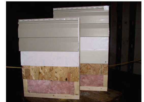
Figure 5. Photograph showing structural differences between unrestricted (left) and fire resistant (right) construction.
