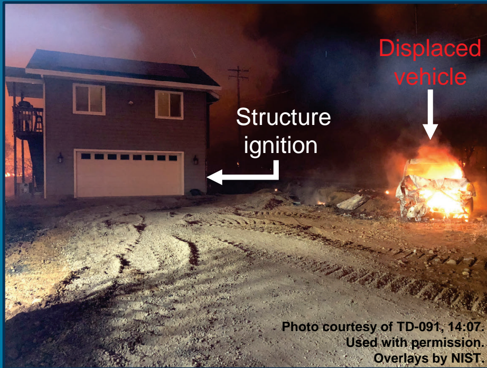
a) A dozer displaced the vehicle to stop fire spread
