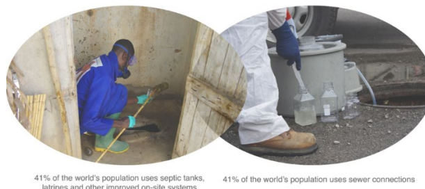
Figure 1. Sample collection methods for pathogens from pit latrines (left) and sewer systems (right).
