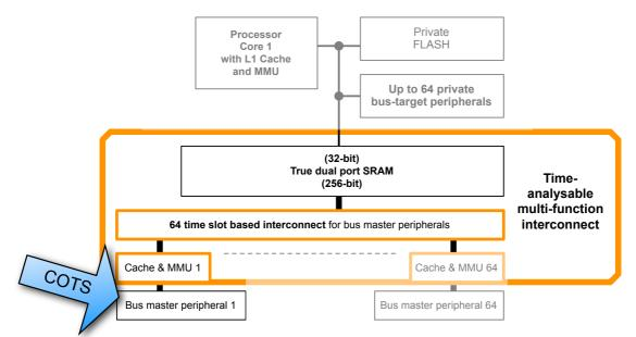
It is trivial to configure SSRT at design-time to ensure that each COTS bus-master peripheral has guaranteed wire-speed bandwidth with low latency
