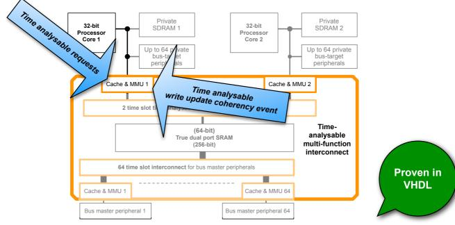
The time analysable memory transfer requests issued by the processor core to the cache of the interconnect experience zero timing interference wrt. all write coherency events issued over that interconnect
