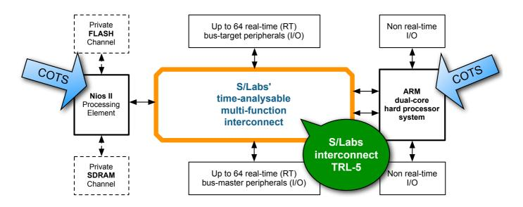
The unmodified Nios II core and COTS peripherals located in the programmable logic of the FPGA experience zero timing interference from the fast unmodified ARM cores and COTS peripherals located in the hard processing subsystem of the FPGA
