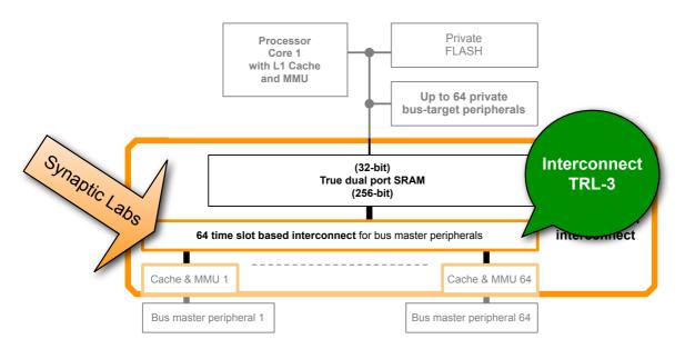
Employs S/Labs' up to 64 time slot based interconnect for bus master peripherals
