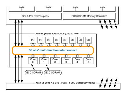
4. Implement our field-proven technology as a hard-macro in a SoC FPGA device or as dedicated ASIC chips
