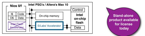
This tiny cache (35 4LUT, 1KB SRAM) informs the commercial development of the tiny caches for bus-master peripherals in SSRT
