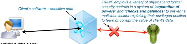
A client of the public cloud A client encrypts sensitive data and sends it to a TruSIP public cloud for processing on the client's software.
