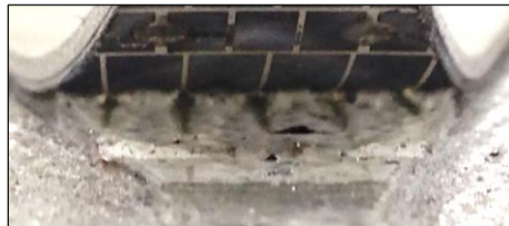
Debond of EVA from cell - localized EVA deformation between grid lines.
