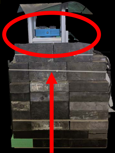
Camera mounted on top of frame
