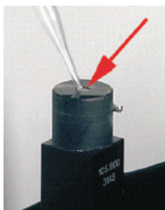
Figure 4. Recessed sample loading window at the top of the nanoCell.
