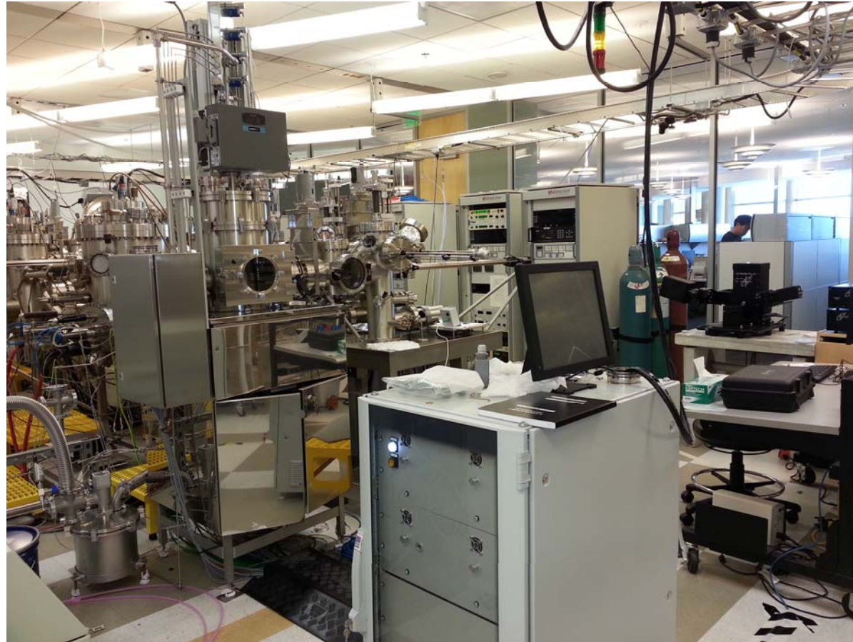
Remote Plasma-Enhanced R200 ALD Reactor at UT-Dallas
