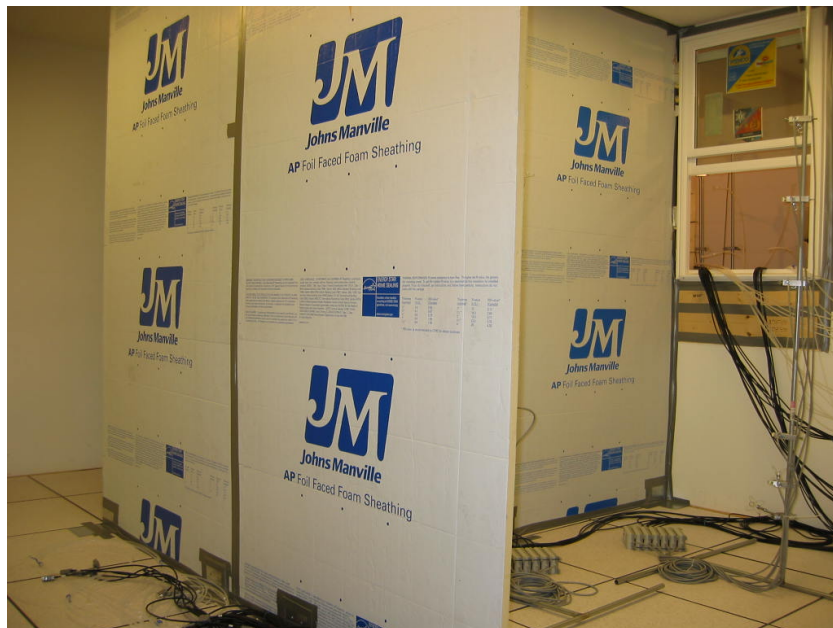
(b) Internal view of the environment chamber partitions inside the test chamber with the partition door removed for each zone
