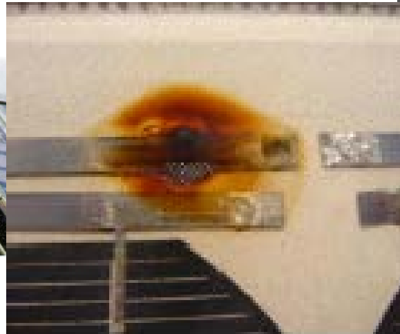
Failed Solder Bond
