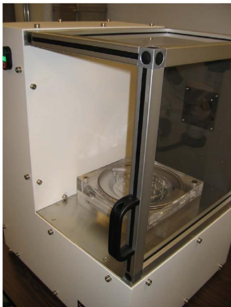
Fig. 2 (left) Chamber ventilation shroud pulled forward. (right) Chamber ventilation shroud moved to back.
